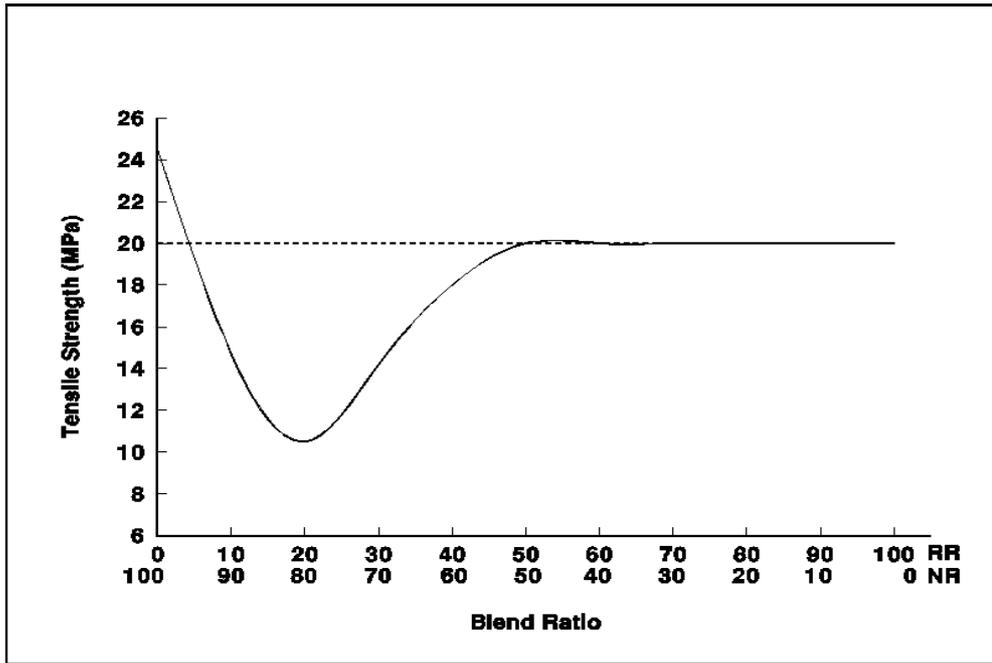
Figure 10. Tensile strength at hardness of IRHD 65 ± 5.
