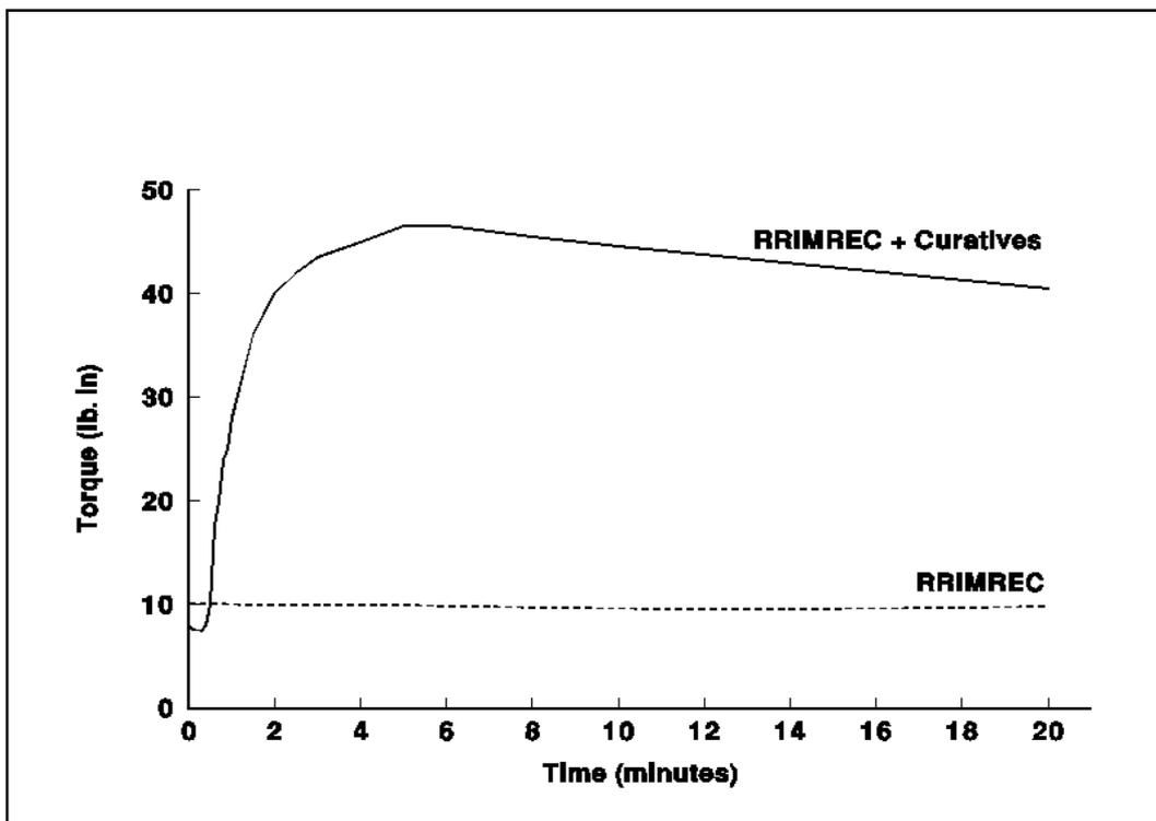
Figure 2. Rheometric traces of RRIMREC.
