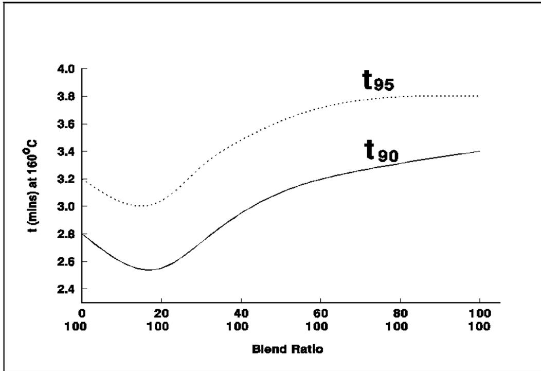
Figure 9. Effect of RRIMREC as fillers on t<sub>90</sub> and t<sub>95</sub>.
