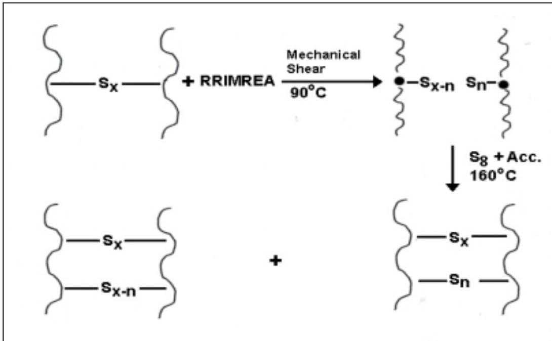
Figure 1. Theory of crosslinking mechanism in RRIMREC process.
