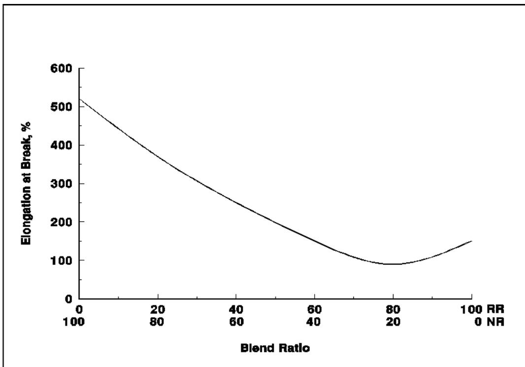
Figure 6. Effect of NR:RRIMREC on elongation at break.
