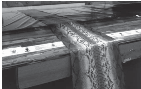
Figure 22: Plating process in an Italian tannery
