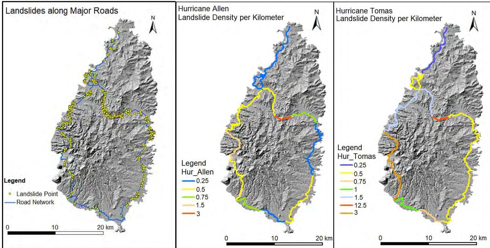
Figure 5-6 Landslide density per Kilometre of Road – Post hurricane Allen (left) and Post Hurricane Tomas (Right)
