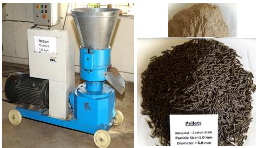
Figure 3. Small size pelletizer and 6 mm pellets prepared from milled cotton stalks
