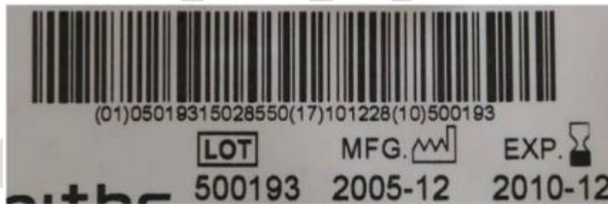
Figure 4-4 Example of a GTIN with additional barcoded information, such as expiration date and lot number
