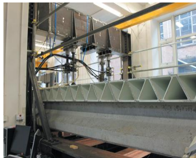
FRP bridge deck
