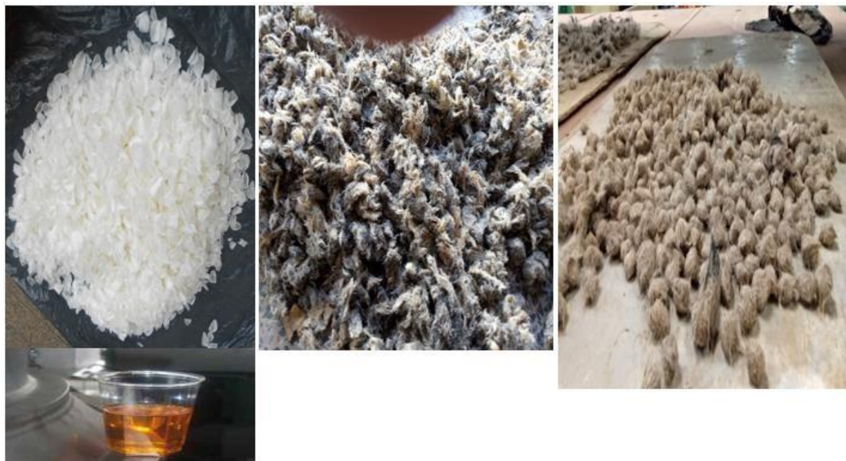
The extracted enzyme solution(left), enzymatic dehairing in process (middle) and recovered hair and scales (right).
