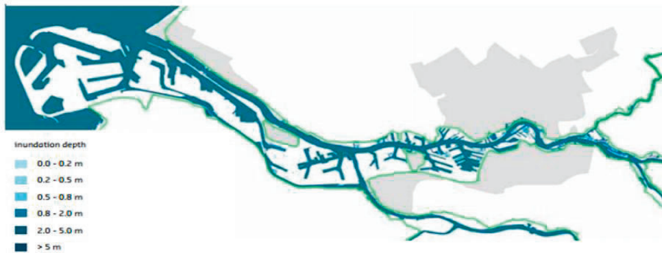
Map 1: Outer-dike flooding in Rotterdam in 2015 (source: Deltares) with a frequency of 1 x 1,000 years
