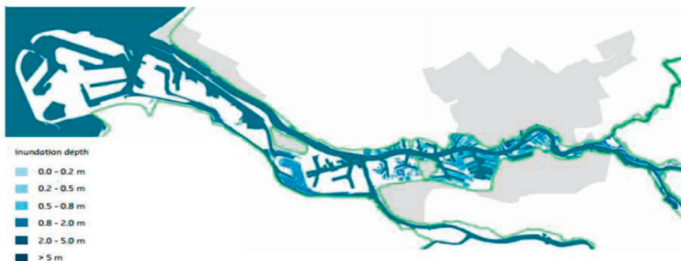
Map 2: Outer-dike flooding in Rotterdam in 2100 (source: Deltares) W+ climate scenario with a frequency of 1 x 1,000 years
