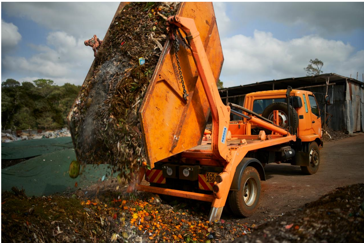
Tipper truck turning organic waste at cycling site for processing into organic fertilizer
