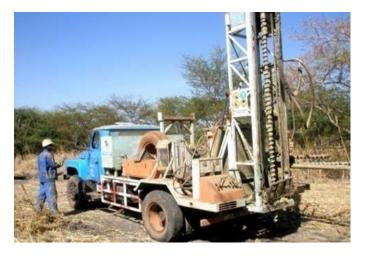
Dongfeng auger rig Drilling Shot hole
