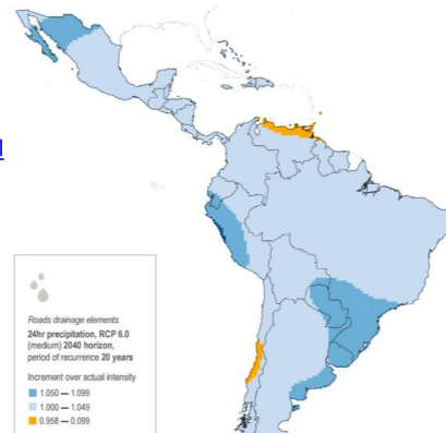
Climate change scenario proposed for roads drainage elements 24-hr precipitation using RCP 6.0.
