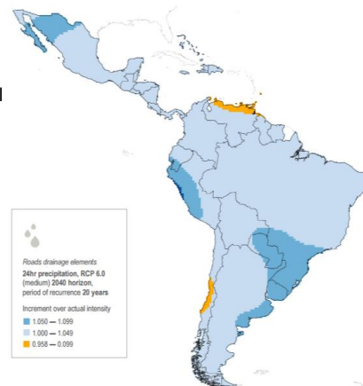
Climate change scenario proposed for roads drainage elements 24hr precipitation using RCP 6.0.
