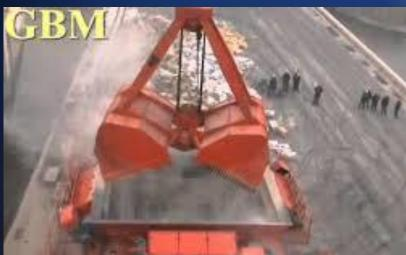
around four side of honory has 4 exhaust inlet, dust will been inhulation to fan from exhaust, thereby can avoid dust.
