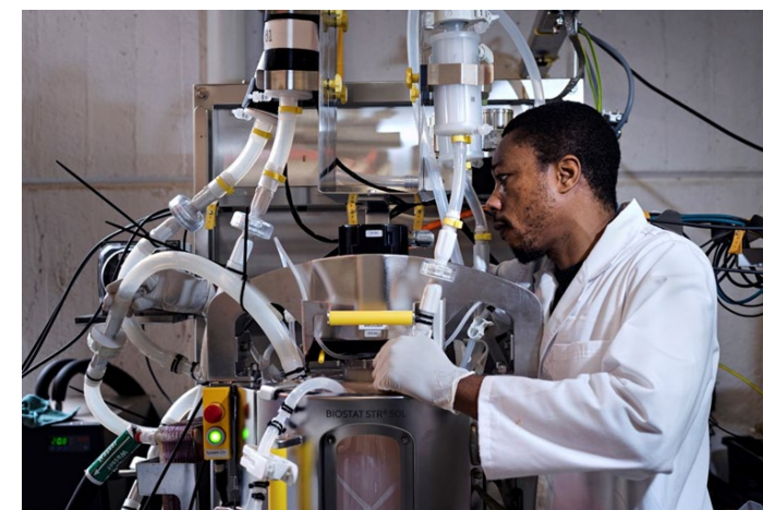
Seaweed fermentation to produce PHAs. Credits: Uluu, 2024
