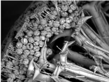
Figure 5.2. SEM image of sterrasters (1) and dichotriaenes (2) in biosilica from Geodia barretti .
