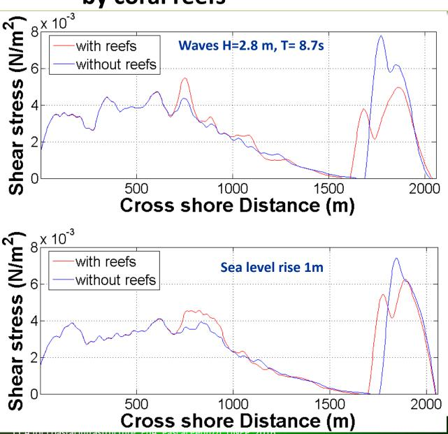
Fig. 9b. Modelled <u>bed</u> <u>shear stress</u> (force per unit area) (SBEACH model) induced by waves in the Negril coastal zone, showing the protection effects of inshore <u>coral</u> <u>reefs</u>
