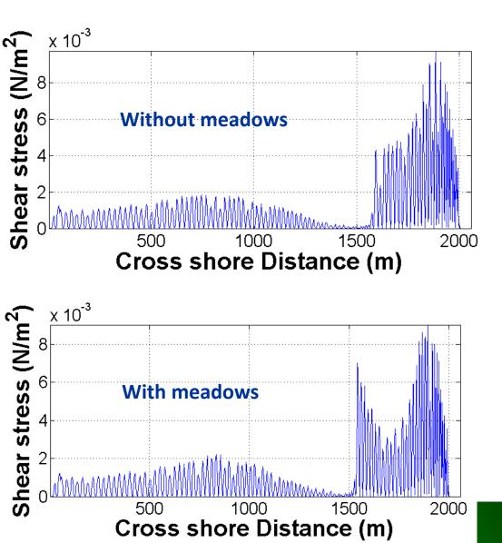
Fig. 11. Modelled <u>bed shear stress</u> (force per unit area) (SBEACH mode (wave height 1 m, period 6s) <u>in the</u> <u>Negril coastal zone</u>
