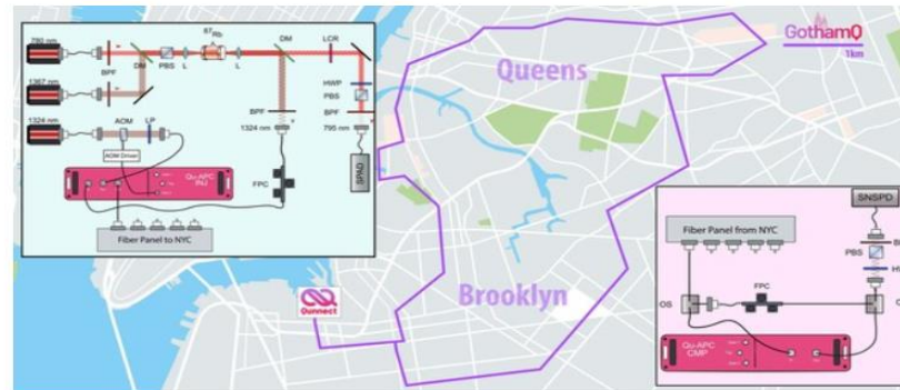
Diagram of the 54 Km GothamQ Quantum Networking Testbed in New York. Credit: Qunnect
