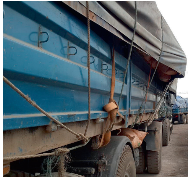
Figure 5.2 An unstable load
