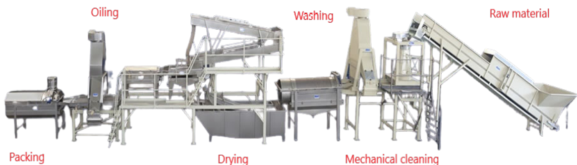
Figure 15. Processing line equipment for dried grapes
