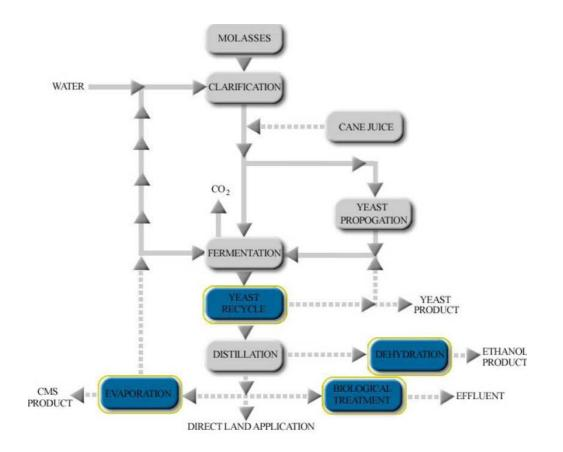
Figure 5. Process flow diagram for manufacture of ethanol from molasses
