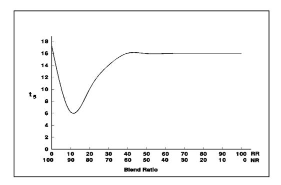
Figure 8. Effect of RRIMREC as filler on t<sub>5</sub>.
