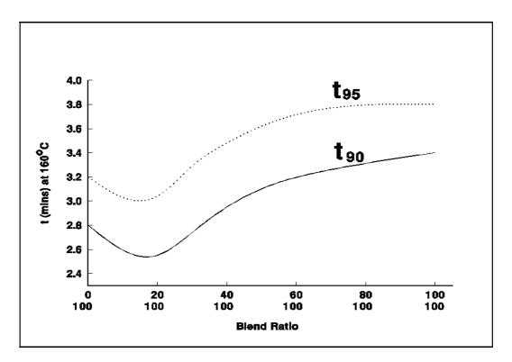
Figure 9. Effect of RRIMREC as fillers on t<sub>90</sub> and t<sub>95</sub>.
