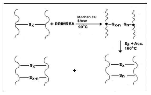
Figure 1. Theory of crosslinking mechanism in RRIMREC process.
