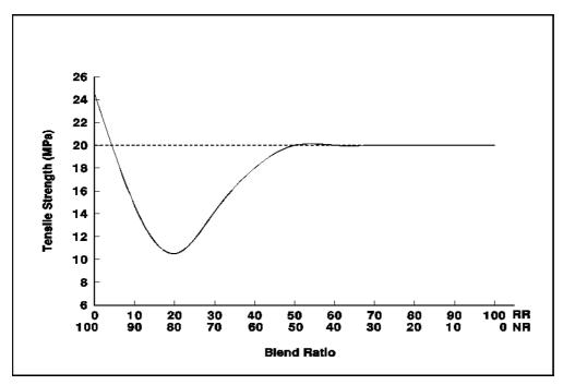
*Figure 10. Tensile strength at hardness of IRHD*  $65 \pm 5$ *.*
