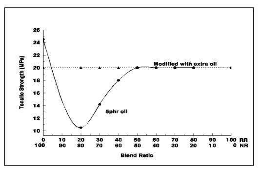
Figure 12. Effect on tensile strength.
