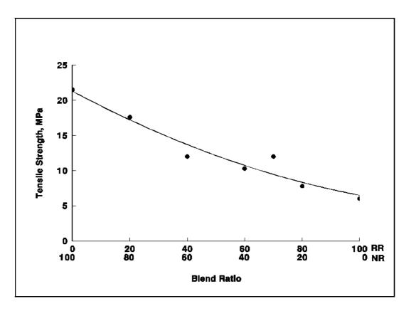
Figure 5. Effect of NR:RRIMREC on tensile strength.
