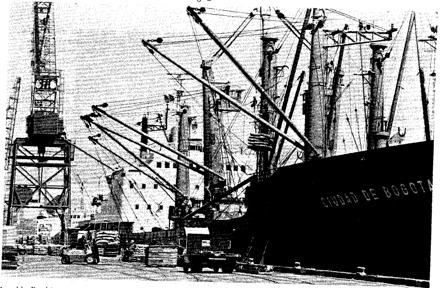
Breakbulk ship at work with 50 ton level luffing crane at standby
